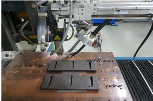
Fig. 2.2 Experimental setup for CO 2 laser-GMA hybrid welding
