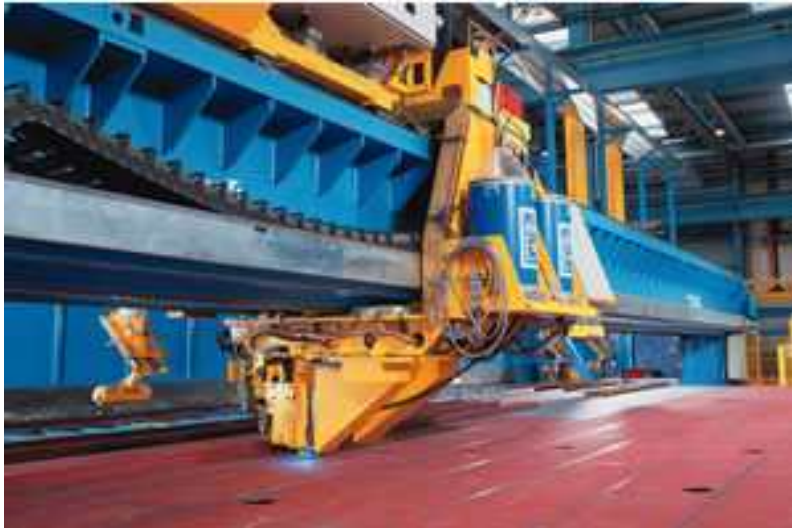
Fig. 1.2 Application example of laser-arc hybrid welding
