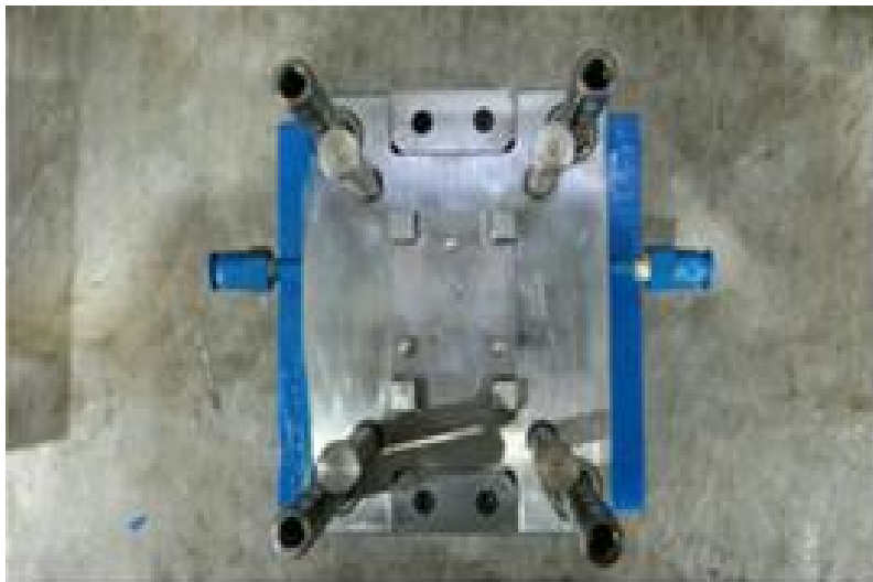
(b) Fabricated fiber guide-plated plan view
