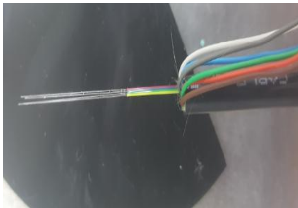
(b) Cable after stripper process
