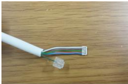
(b) Hybrid cable after socket squeeze process is complete
