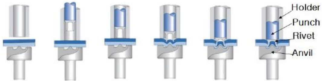
Fig 1.8 Organizational tree of self-piercing rivet process
