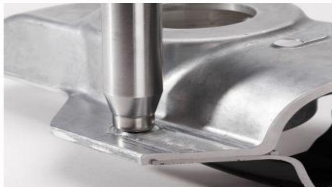
Fig 1.7 Friction spot joining process
