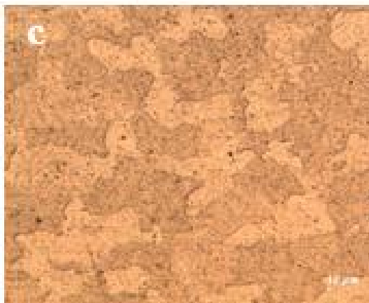
Fig. 3.2 Microstructure of FSW welded joints at y-axis tilting angle 1^\circ (a:SZ, b:TMAZ, c:HAZ, d:BM)
