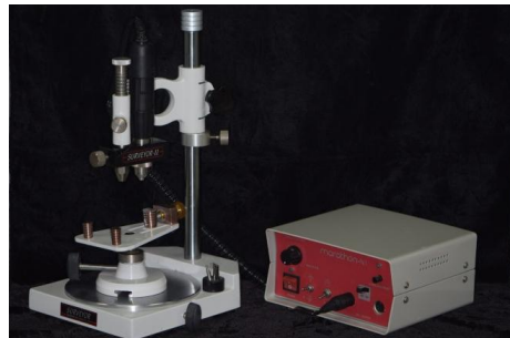
Fig. 2. Surveyor with surgical drill and engine.
