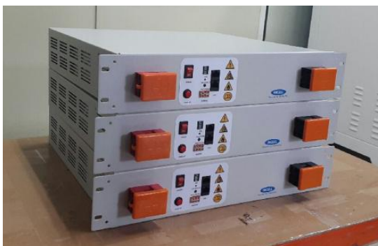
Fig. 4-1. Screening-based energy storage system (14S20P)
