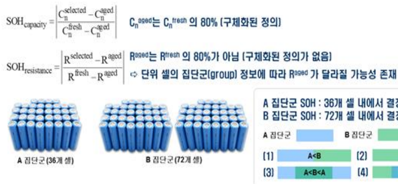
Fig. 4-13. Resistance-based SOH measurement according to cell group
