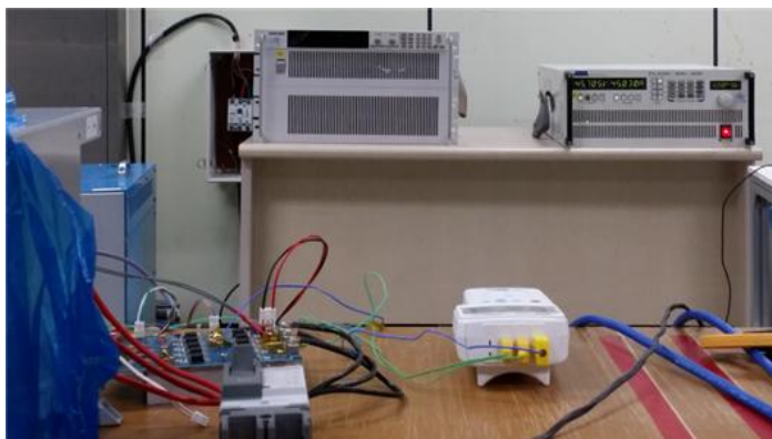
Fig. 3-30. Protection circuit module(above a rated current of 30A)
