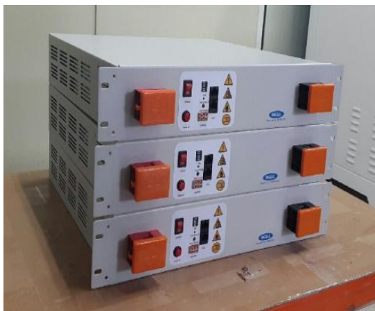
Fig. 3-9. Screening-based energy storage system(14S20P)
