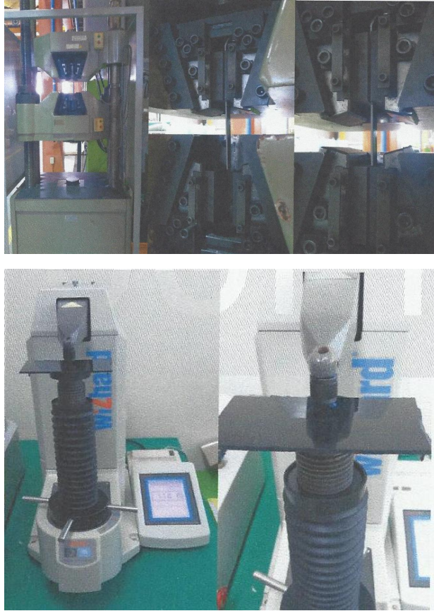
Photo. 3.3 Test equipment of HRR hardness and tensile strength
