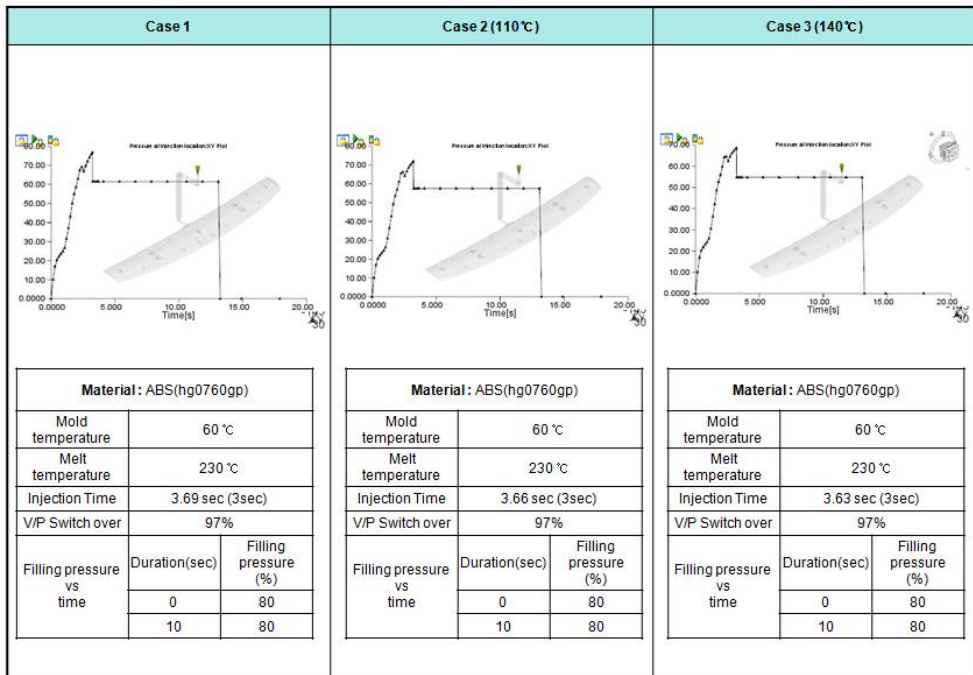
Fig. 4.4 Injection flow analysis to the cavity temperature
