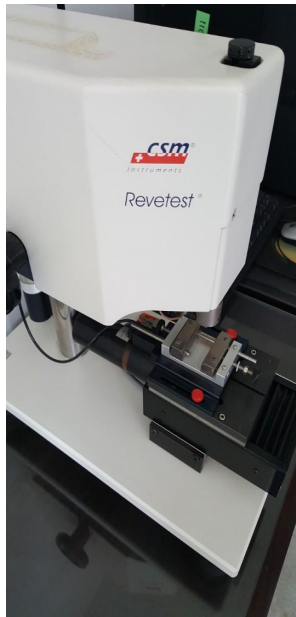
Photo. 3.2 Scratch test equipment
