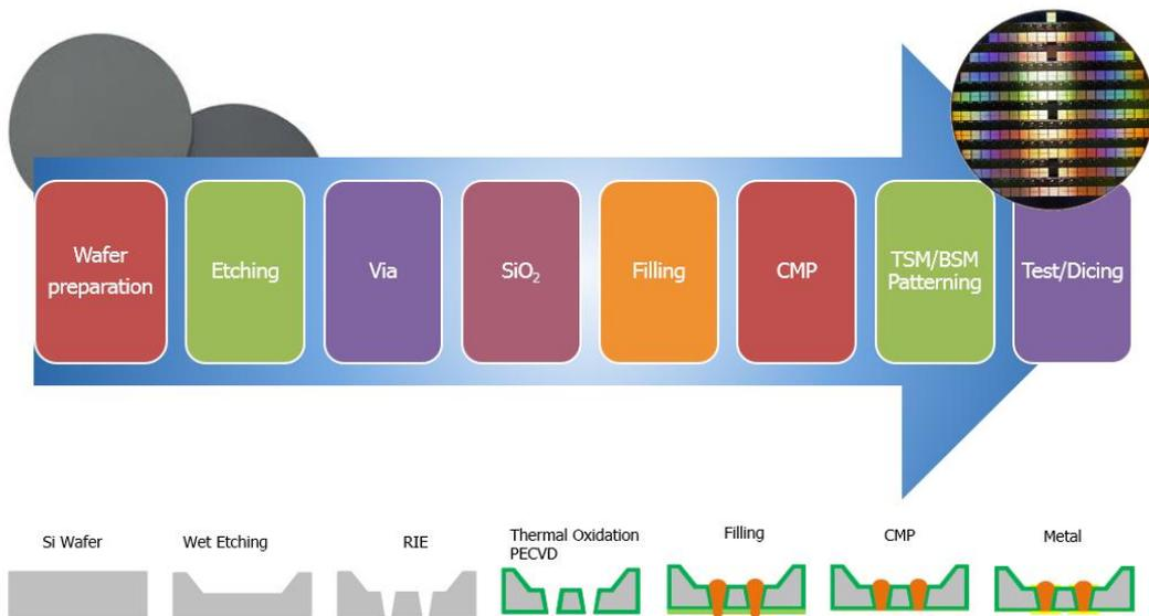
**Fig. 2** Silicon Electrical Circuit Board manufacturing process
