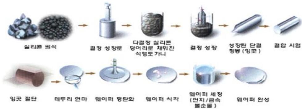
Fig. 5 Silicon Wafer Manufacturing Process
