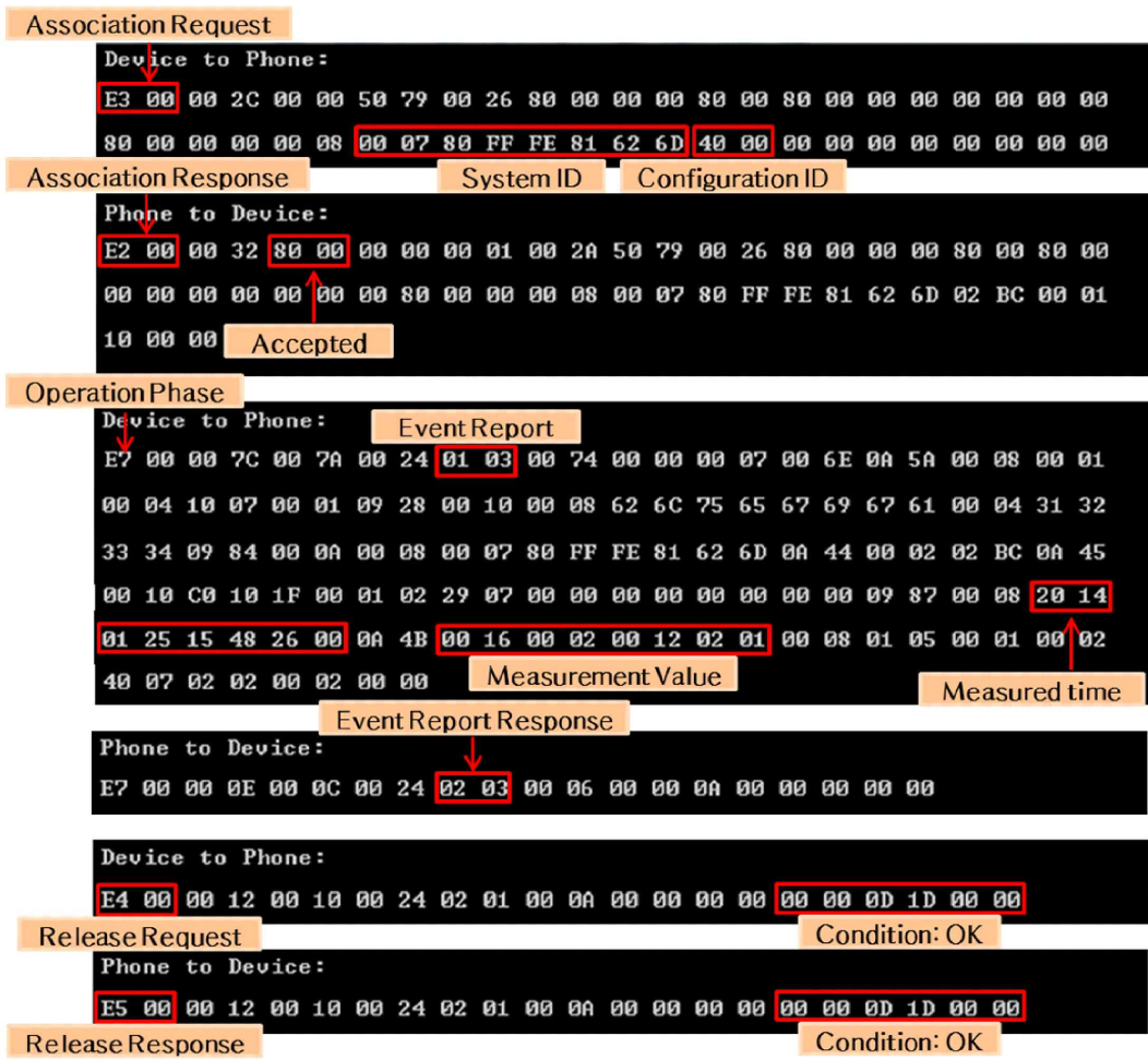
Figure 2.13. ISO/IEEE 11073 messages exchanged between PHD agent and PHD manager.
