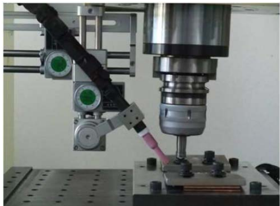
(b) Experimental setup for TIG assisted hybrid friction stir welding (HFSW)
