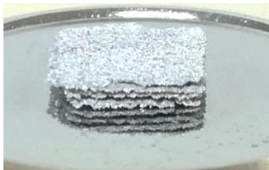
Fig. 71 Delamination of the fabricated part through multi-layers deposition (without heating of building plate)
