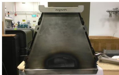
Fig. 8 Thermal shielder of EBM process (ARCAM AB)
