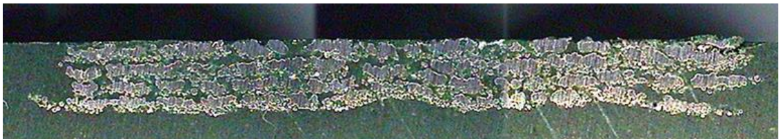
Fig. 72 Morphology of the fabricated part through multi-layers deposition (cross section, without heating of building plate)
