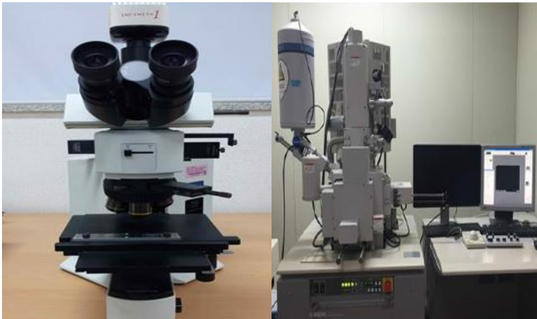
Fig. 2.7 Optical microscope and scanning electron microscope
