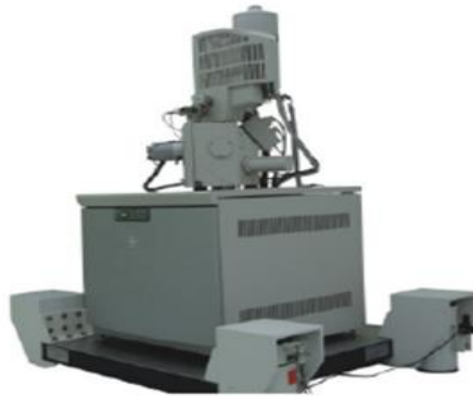
Fig.25 FE-SEM (Field Emission Scanning Electron Microscope)
