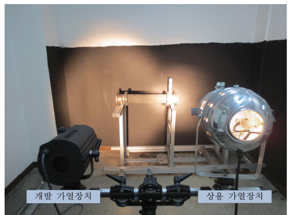
Fig. 3-3 Comparison of illuminance and irradiation range of commercial heating device and developed heating device
