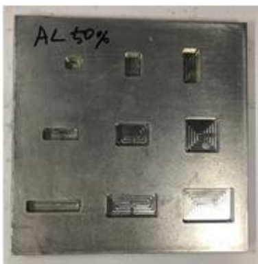
Fig. 4-3 Wall thinning defect specimen(10 mm, 50 %)
