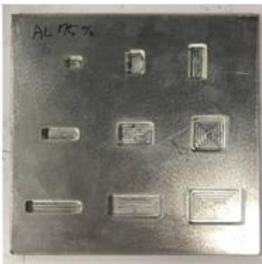
Fig. 4-2 Wall thinning defect specimen(5 mm, 75 %)
