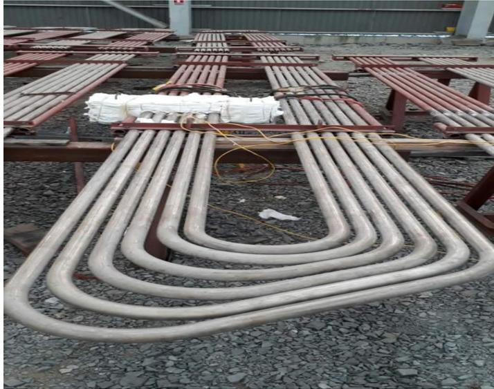
Fig.8 General PWHT of Tube Condition for 120min
