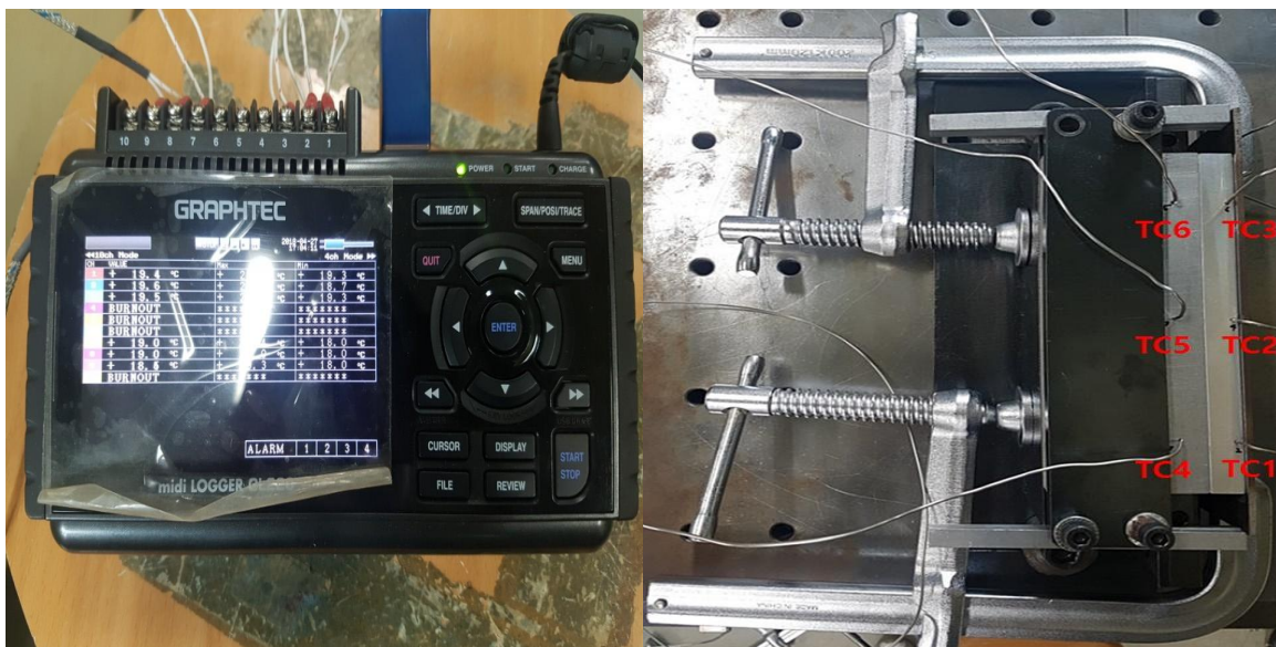
Fig. 2.7 Set up for temperature measurement
