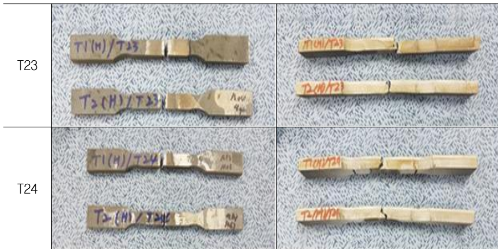
Fig. 3.4 Fracture tensile test specimens for welding conditions of T23 and T24
