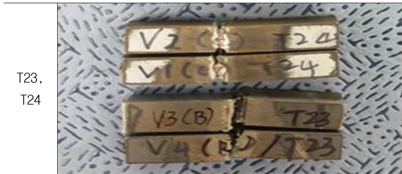
Fig. 3.6 Fracture impact test samples at different welding conditions of T23 and T24
