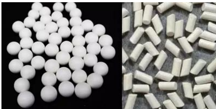
Figure 13. Shape comparison of gamma-alumina sphere and pellet
