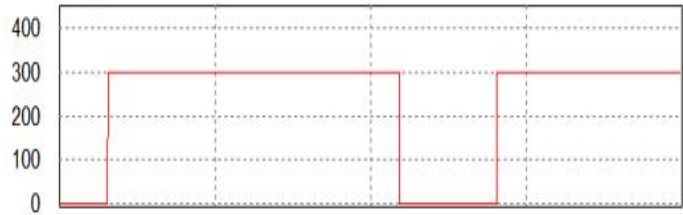
(a) Switch S_a voltage ( V_{ds-sa} )
