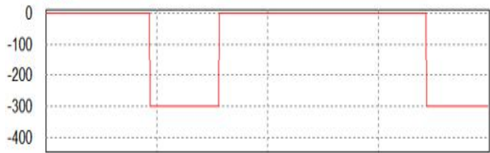
(c) Diode D_1 voltage ( V_{D1} )
