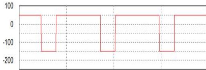
(a) Voltage across inductor L_1 ( V_{L1} )
