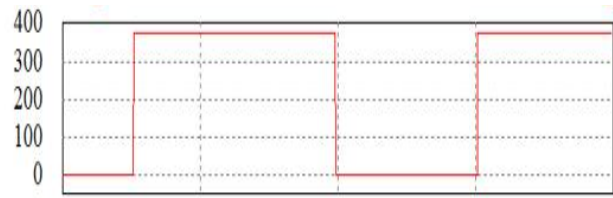
(a) Switch S_a voltage ( V_{ds-sa} )
