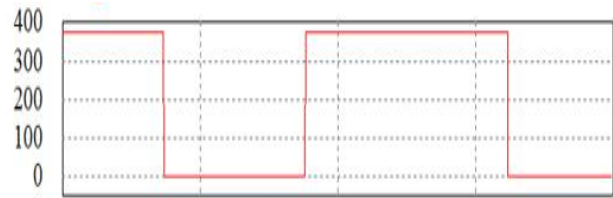
(b) Switch S_b voltage ( V_{ds-sb} )
