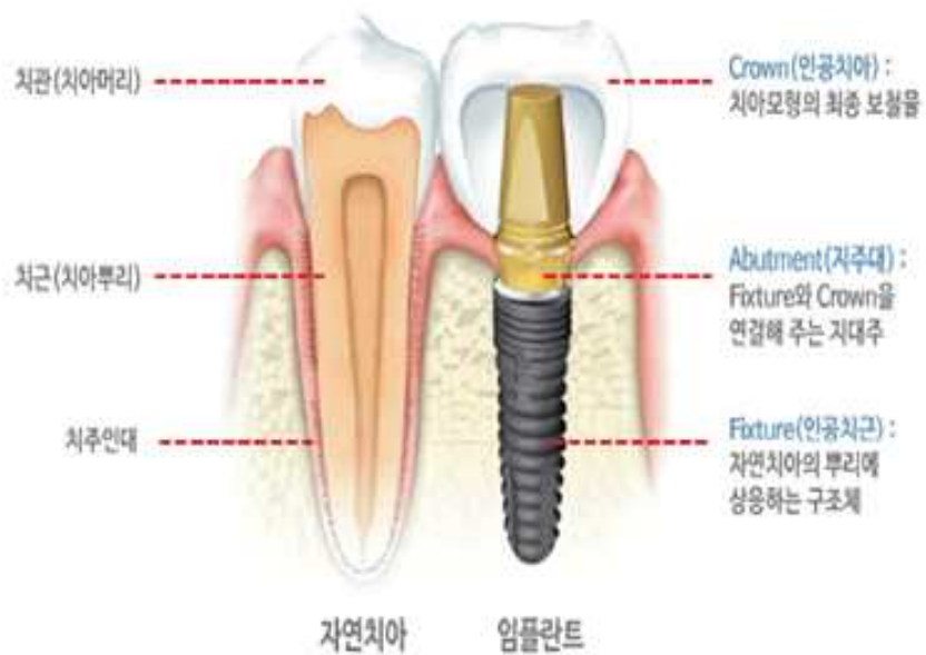
Fig. 2-1. Natural human tooth and Dental implant structure
