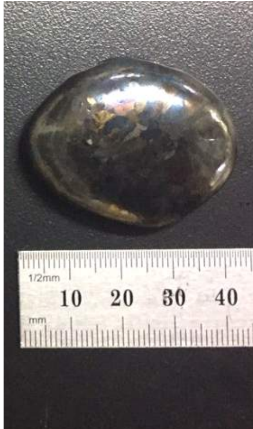
Figure. 3-1. Ingot test specimen of the zirconium manufactured by arc melting furnace in this study
