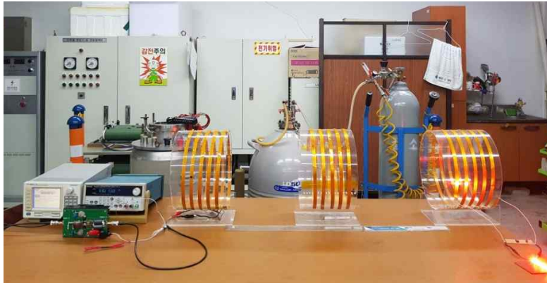
Fig. 4-36 WPT experiment applying the relay antenna
