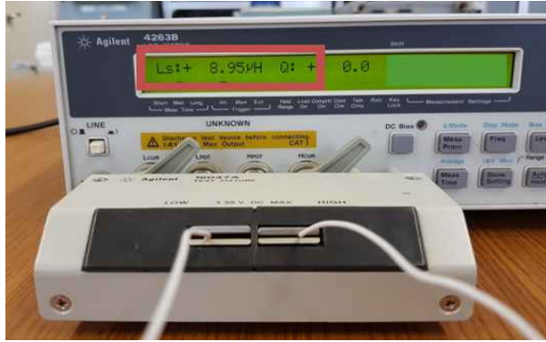
Fig. 3-10 Measured value of the inductance using RLC meter
