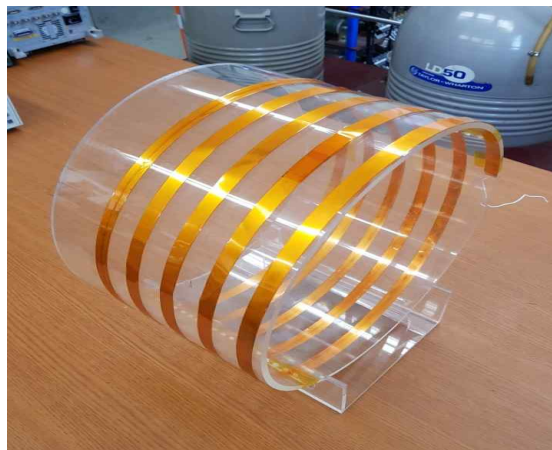
Fig. 3-22 The superconducting relay antenna
