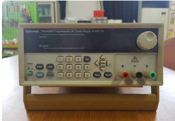
Fig. 3-28 DC power supply
