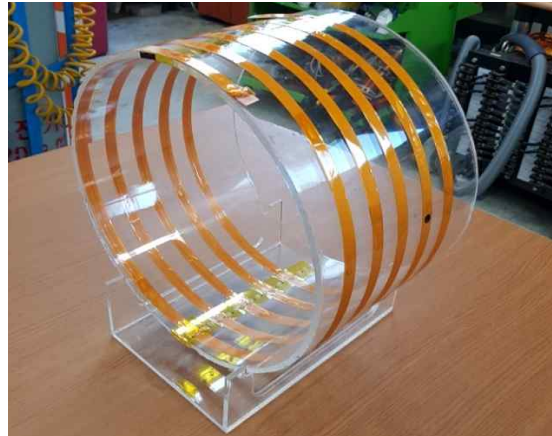
Fig. 3-9 Experimental design of the superconducting helical antenna
