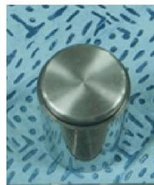
Fig. 2.3 Tool details used for friction spot joining
