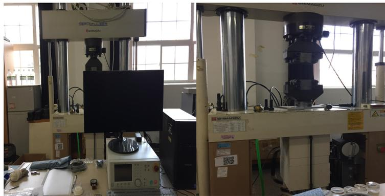
Fig. 2.6 UTM(Universal Testing Machine)
