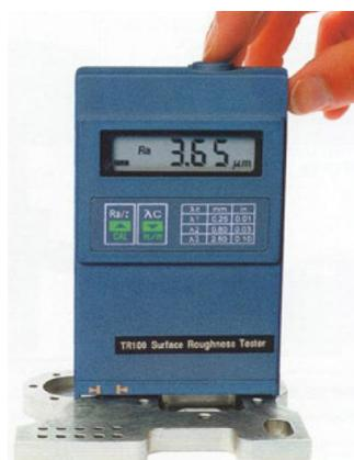
Fig. 2.4 Surface roughness measuring instrument
