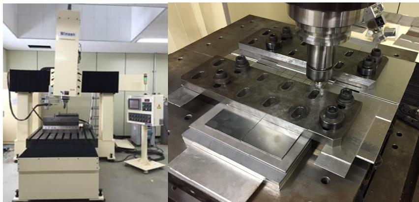
Fig. 2.2 Equipment of friction stir welding system
