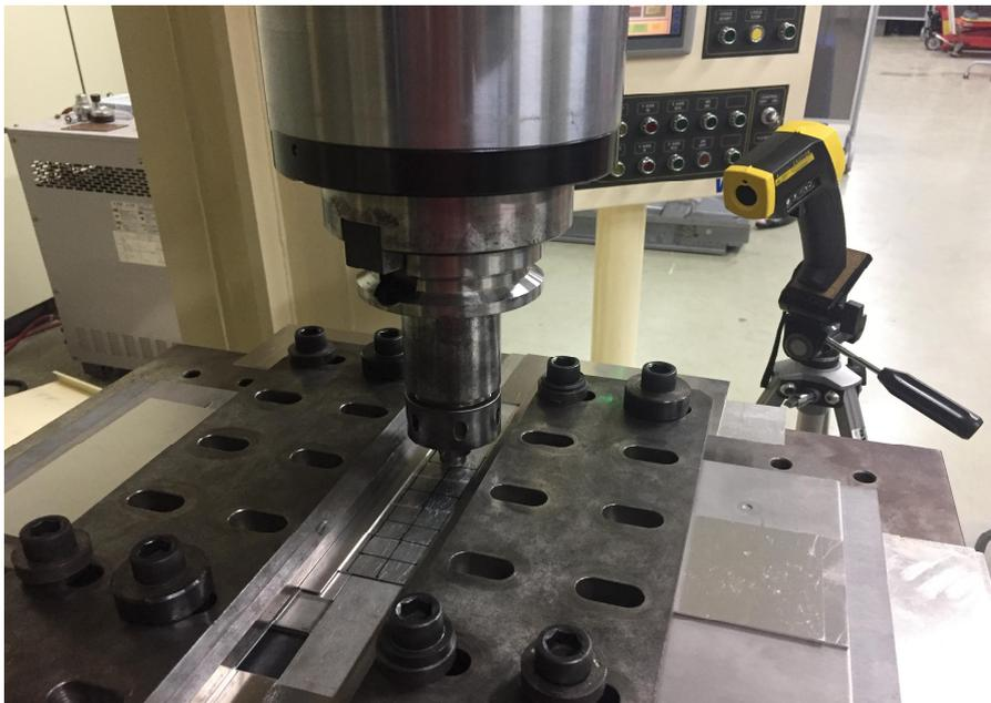
Fig. 2.5 Infrared radiation thermometer
