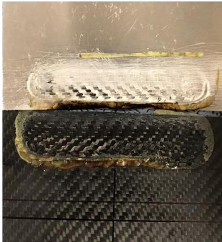
Fig 3.4 Shape of fractured surface of Al/CFRP joints
