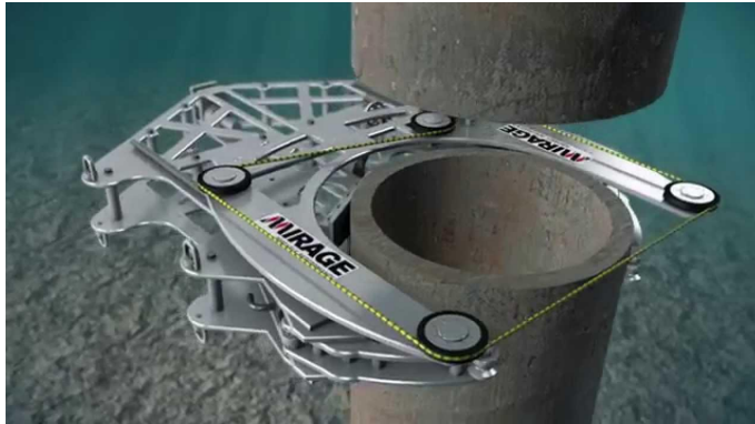
Fig 16. Diamond Wire Saw Cutting
