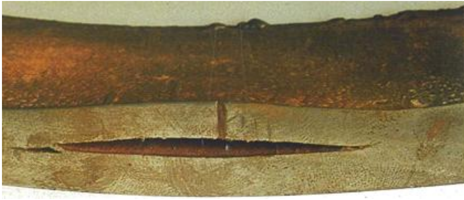
Fig. 2.8 Cross section of a failed sample by hydrogen embrittlement cracking.
