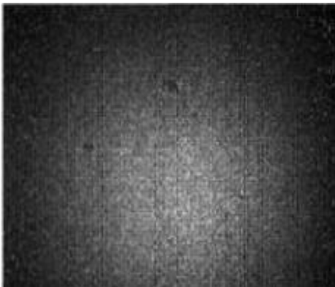
Fig. 2-1 Speckle pattern before the deformation
