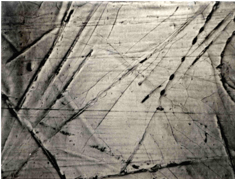
Fig. 5-3 Swelling of glass fiber ends
