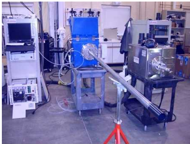
Fig. 2-14. Configuration of Continuous Emission Monitoring System, CEMS.
