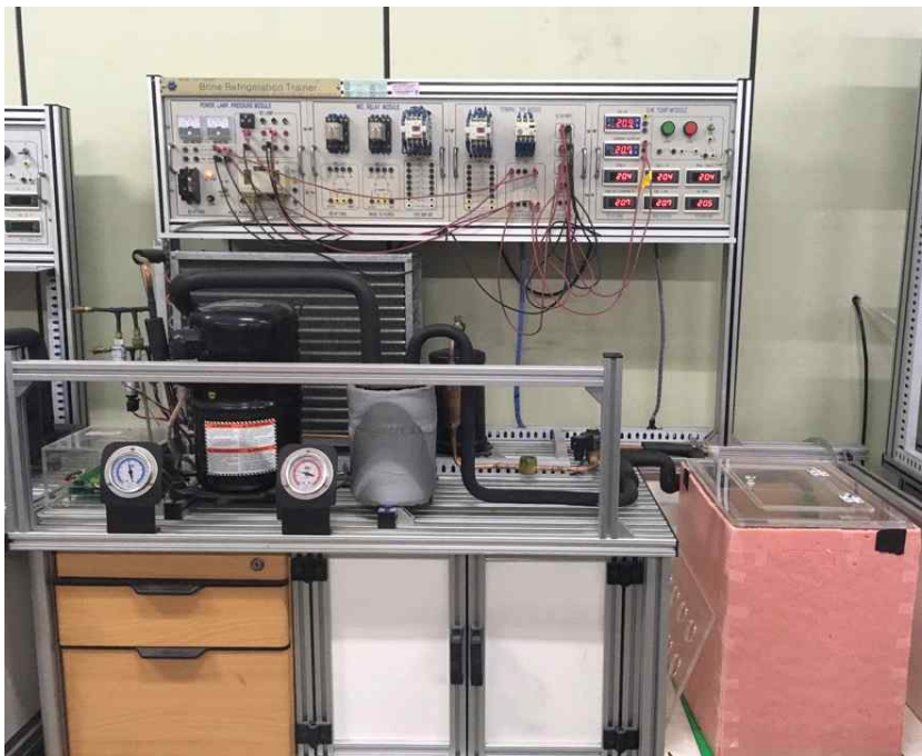
Figure 2.4 A brine refrigeration apparatus used for T-history experiments
