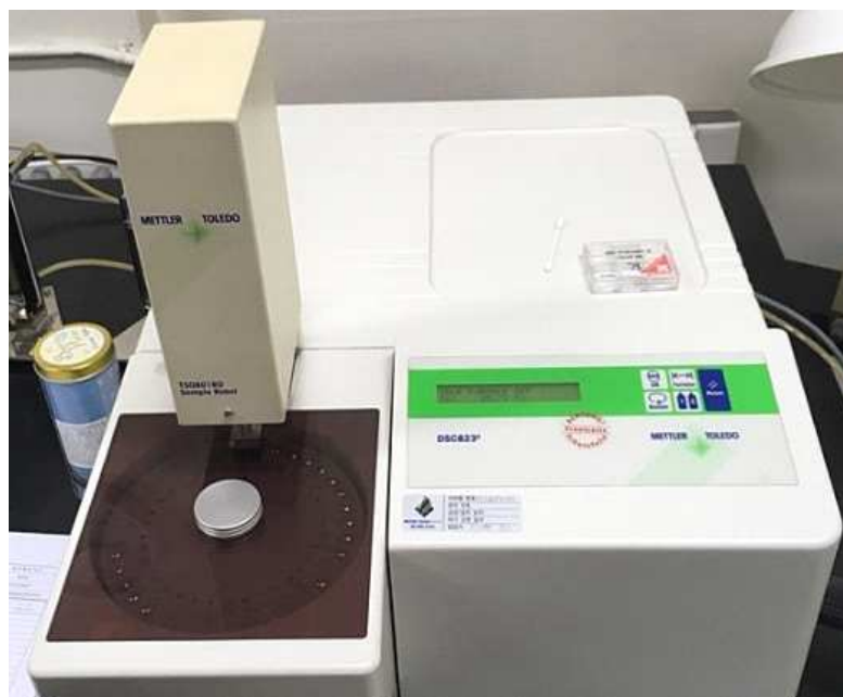
Figure 2.2 Heat flux type DSC used in present the study
