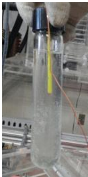
Figure 2.6 K-type thermocouple installation onto the Pyrex test tubes
