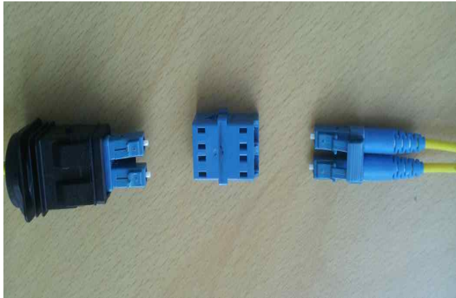
Fig. 2-3 Image of destructive analysis 2(Harting社)
