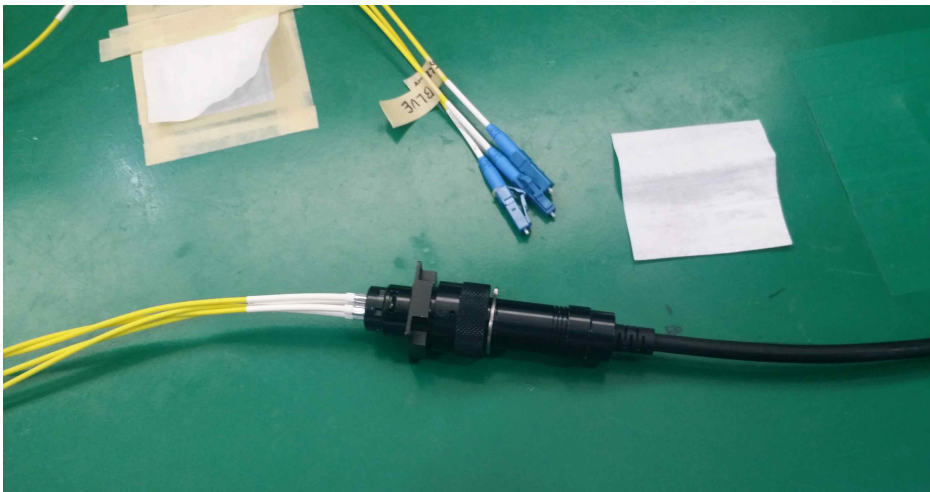
Fig. 2-41 Prototype production of LC Quadplex(a'ssy)
