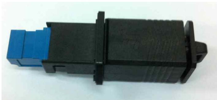
Fig. 2-25 Prototype production of QDM A'ssy(Juction)
