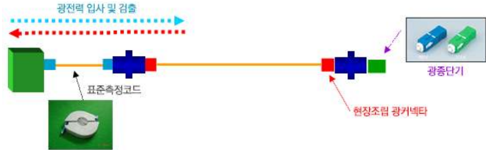
Fig. 1-9 Optical loss measuring device(insertion loss)
