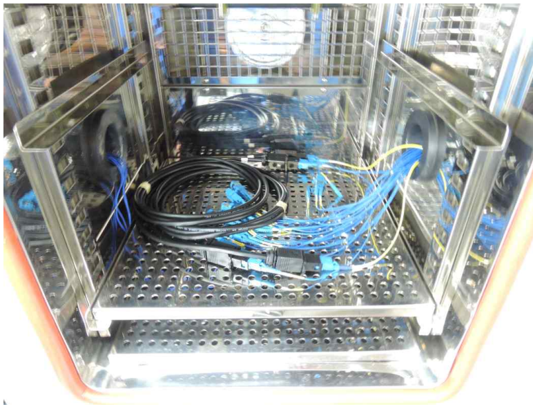
Fig. 3-15 Inside image of temp. cycle test chamber
