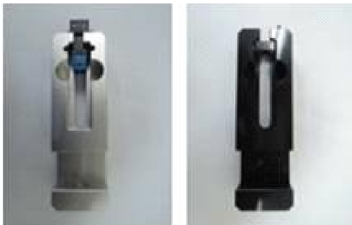
Fig. 3-9 Tensile test jig(assembly)
