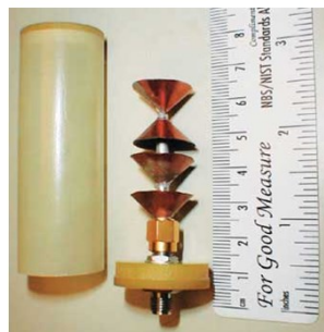
Figure 2.3: Inverted biconical antenna prototype [12]
