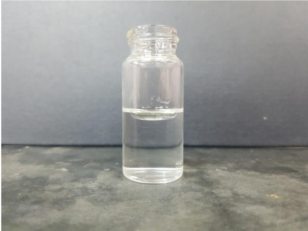
Fig. 9. Image of KJ-001 applied into PBS. Five min after the addition of KJ-001 into PBS, KJ-001 clumped into one place and showed a gel shape.
