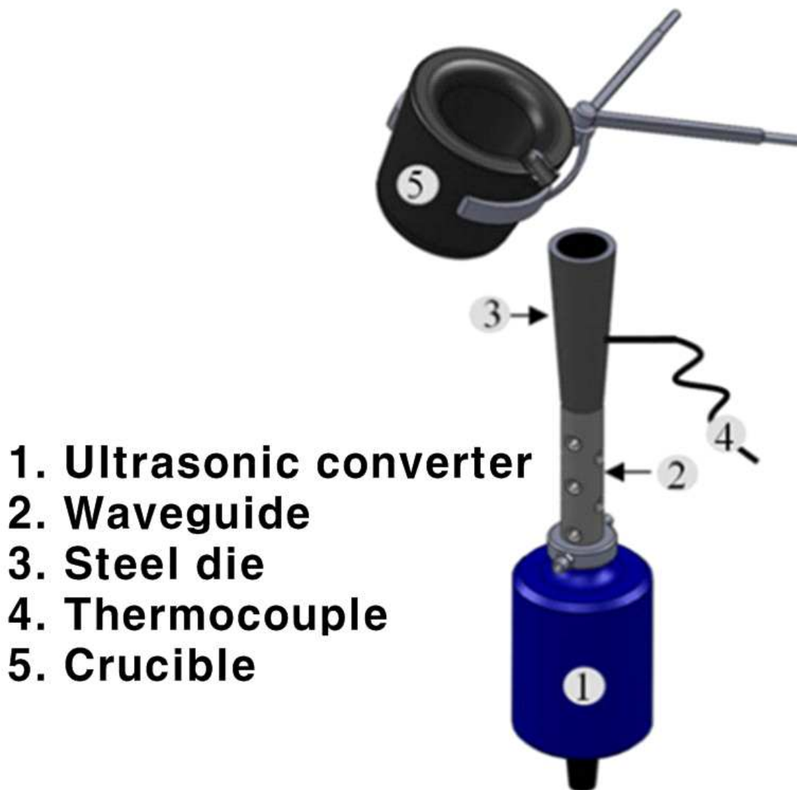
Figure 2.10 Schematic diagram of the ultrasonic converter equipment [52].
