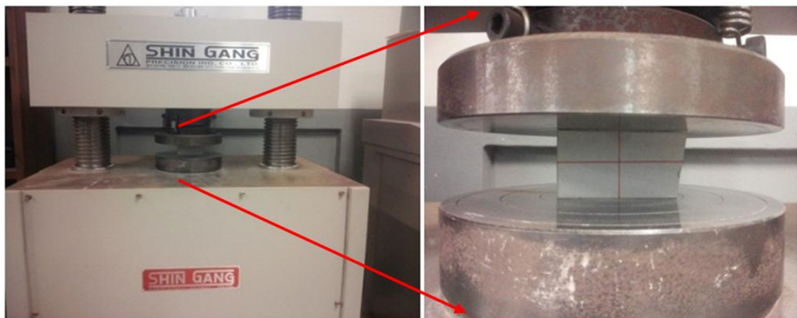
Figure 3.3 Compressive strength test setup
