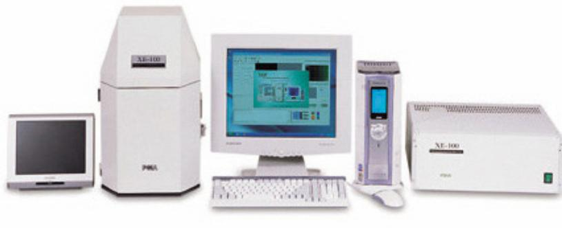
**Fig. 2.** Atomic force microscope for surface roughness measurement.
