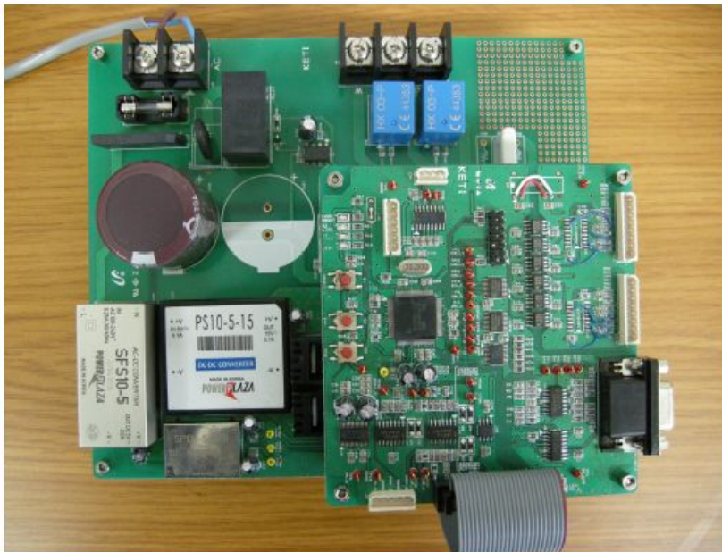
Fig. 3.30 Control device of BLDC motor
