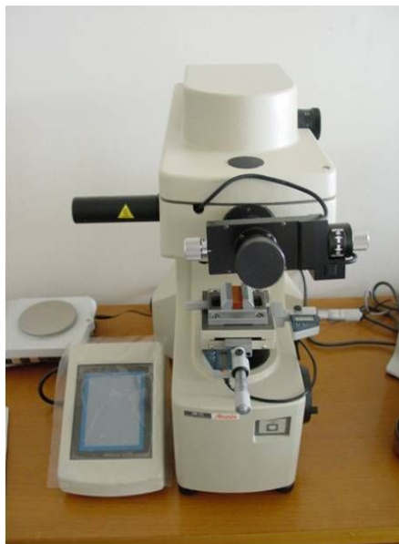
Fig. 2.8 Vickers hardness test scheme and equipment
