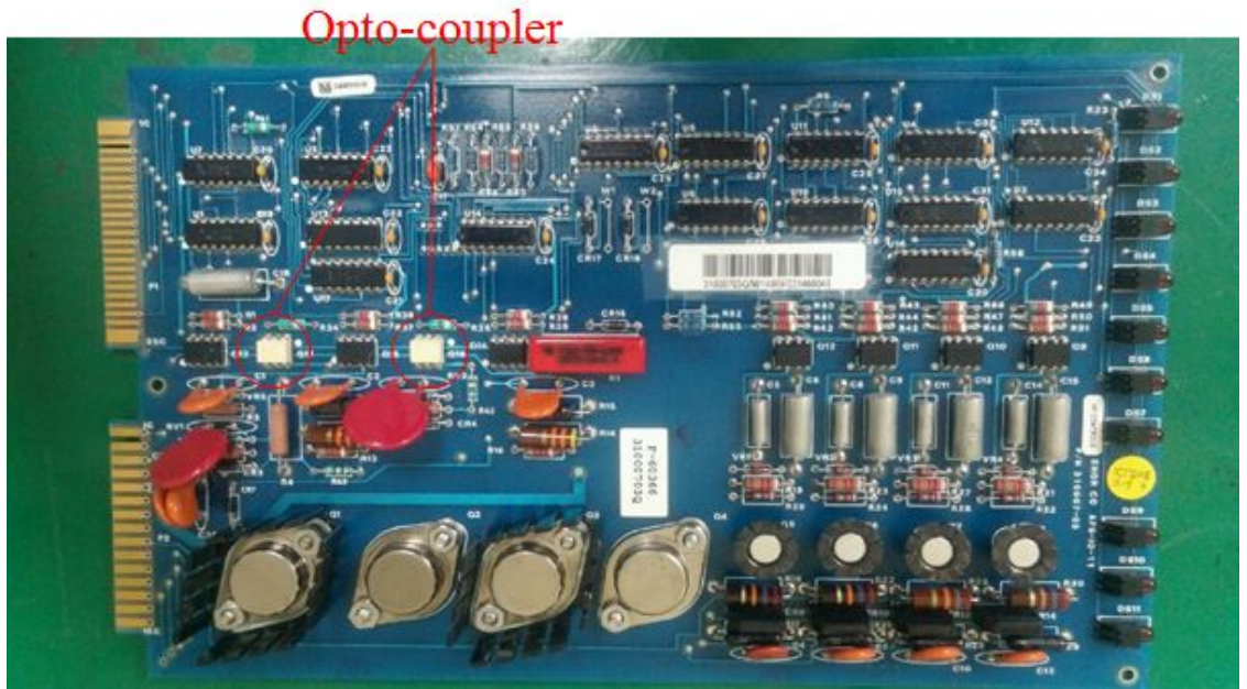
Figure 12. Opto-coupler in the I/O-11 Board
