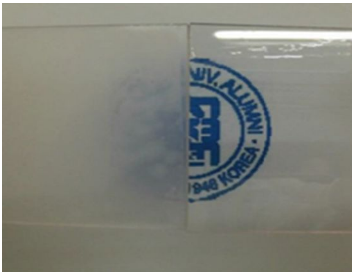
Figure 4.4 Cold anti-fog test of uncoated PC(left) and AF-AO 3 coated PC(right) after removal from -20 °C freezer to humid environment.
