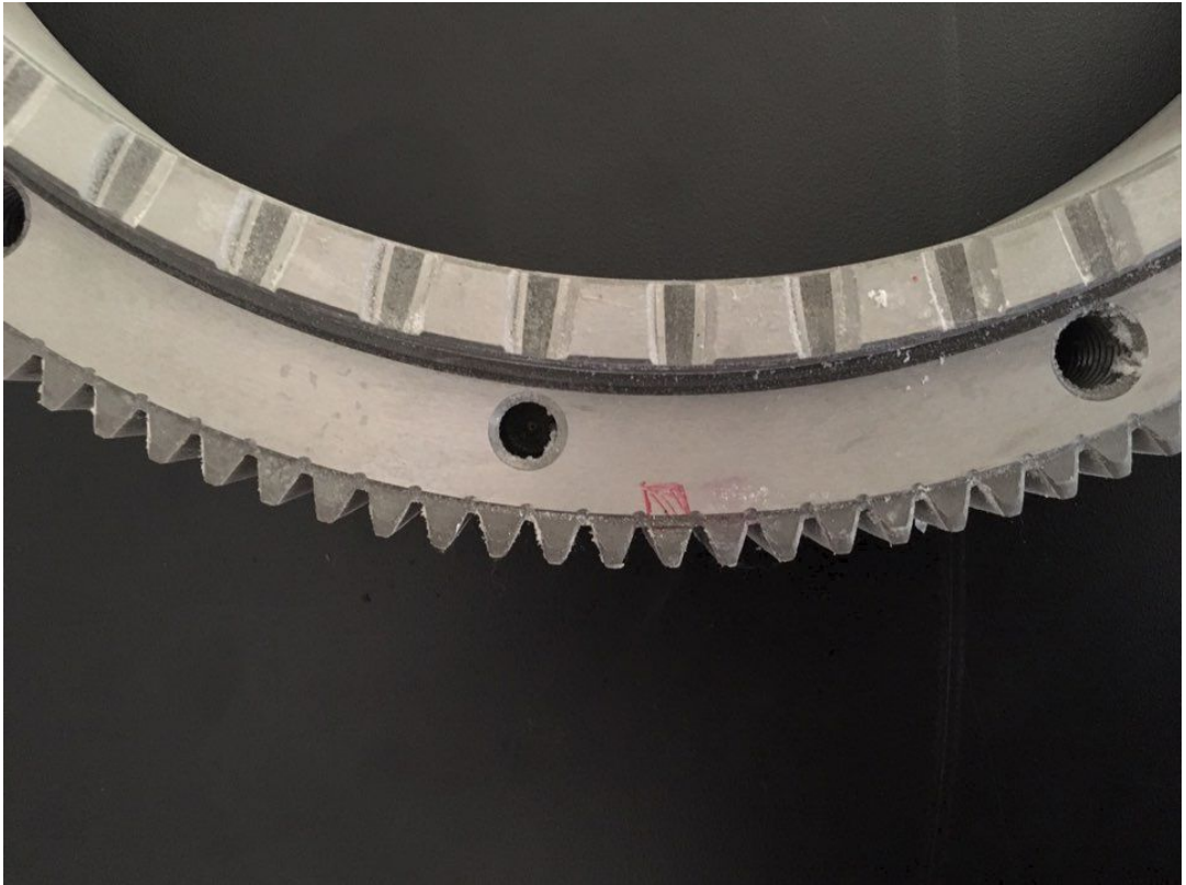
Fig. 5-4 Hybrid CURVIC gear artificial defect specimen
