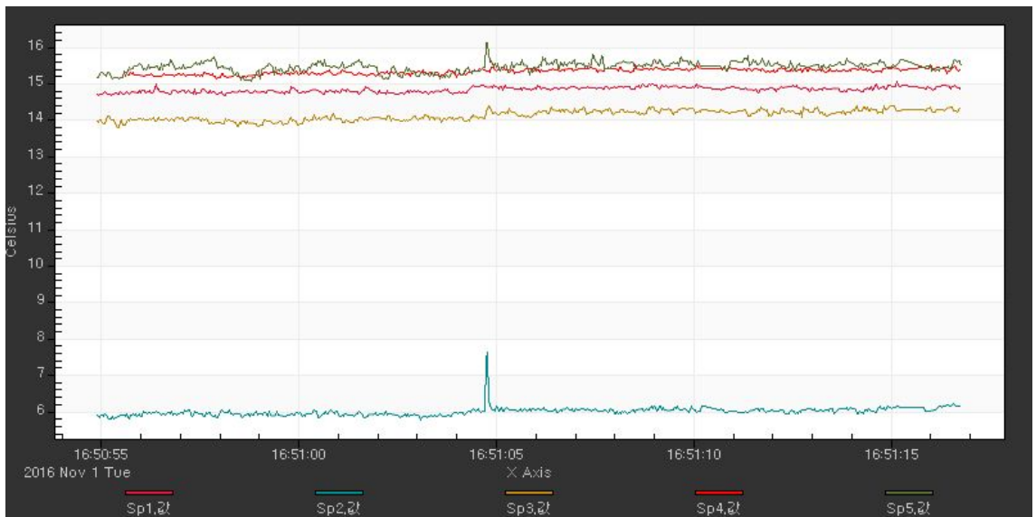
(b) the resulting graph of the temperature of the thermal test hybrid gear after cooling
