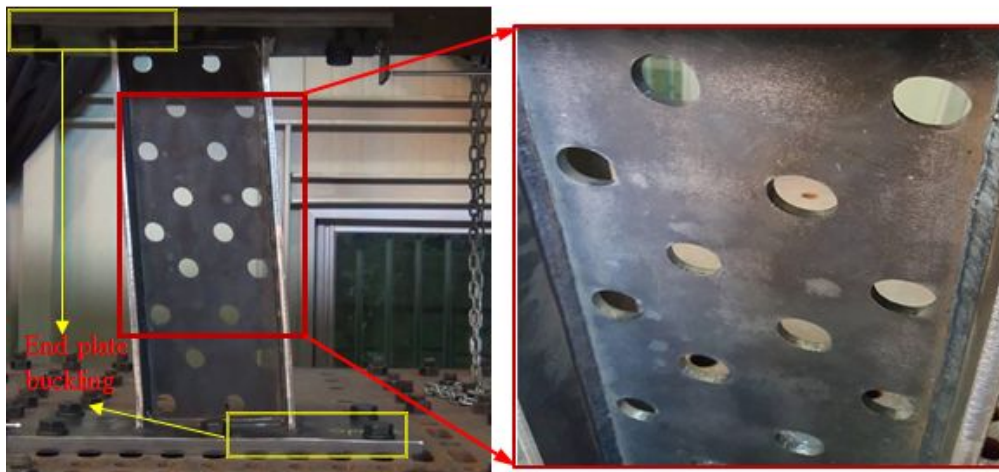
Fig. 4.16 Deformed shape and cracks observed on RWS-U10Sf1
