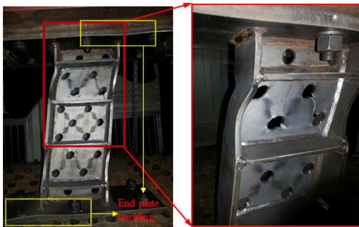
(a) buckling and crack of RLS-S10Sf1
