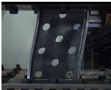
(a) buckling and crack of RWS-U10S1
