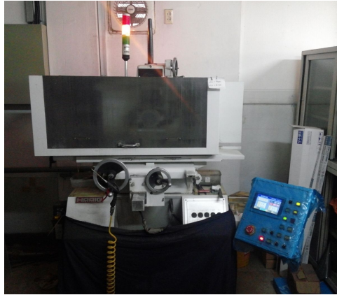
Fig. 2. Slicing machine used to cut blocks into specimens.
