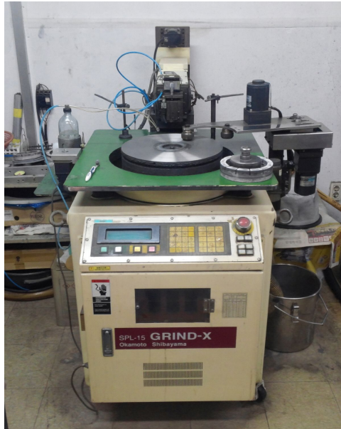
Fig. 3. Lapping machine used for polishing the specimens.
