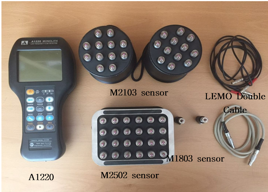
Figure 2-2. Components of low-frequency ultrasonic flow detector.
