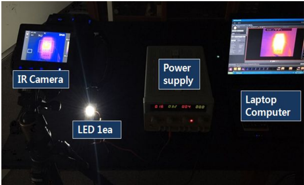
Fig. 3-8 LED chip 1EA for thermal imaging camera temperature measurement
