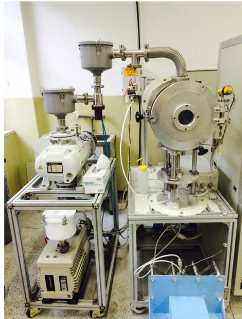
Fig. 8. Apparatus for room temperature spray coating.
