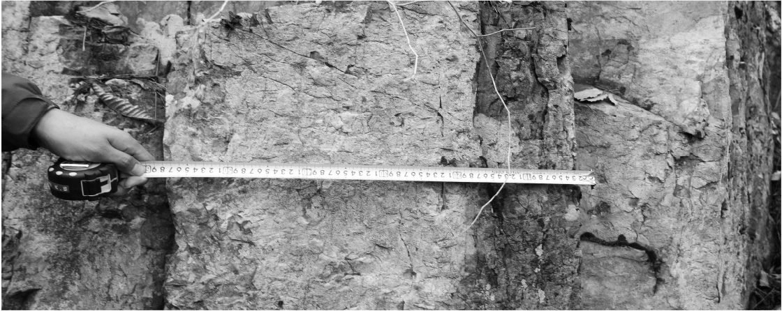
Fig. 40. Photograph of measured columnar joints in BS-09.
