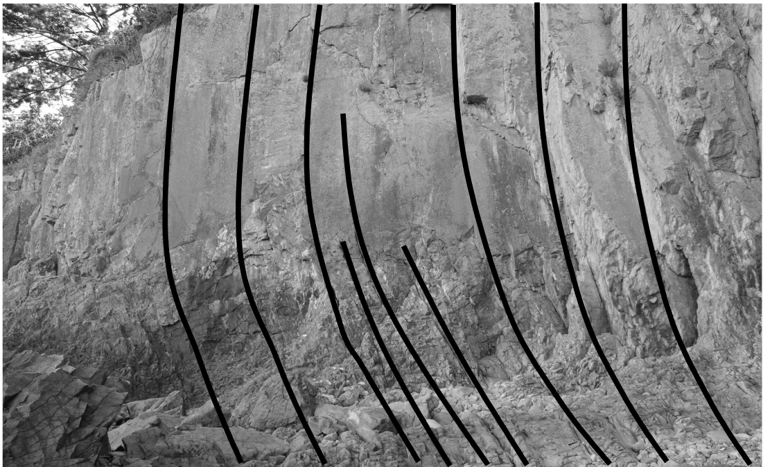
Fig. 29. Photograph of columnar joints in BS-25. (Line is joints)
