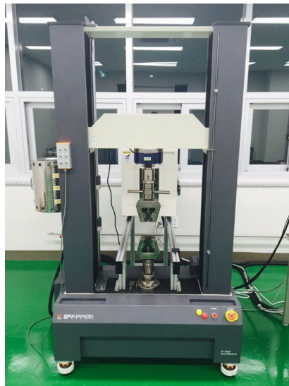
Fig 3.10 Universal testing machine
