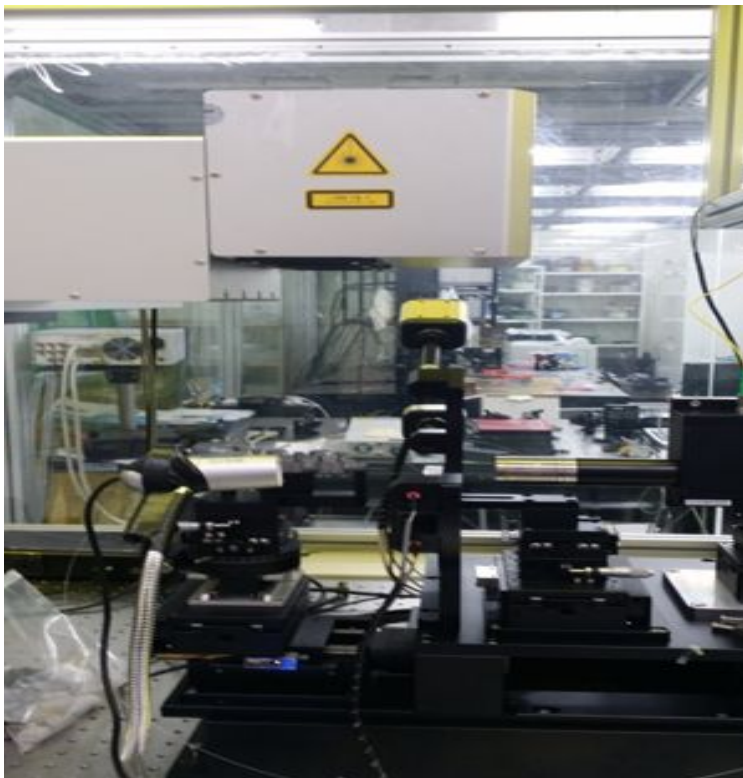
[Photo. 4.2] CO 2 Laser machine used for fabricating quartz specimen with a CO 2 spot
