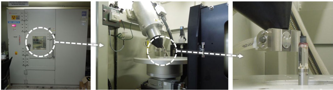
Fig. 55 Micro-focus X-ray computed tomography system
